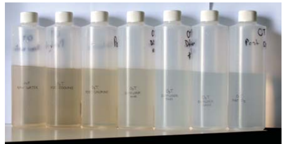
Ammonia, DOC, colour and odour removal and microbial disinfection, for Wanganui DC.
